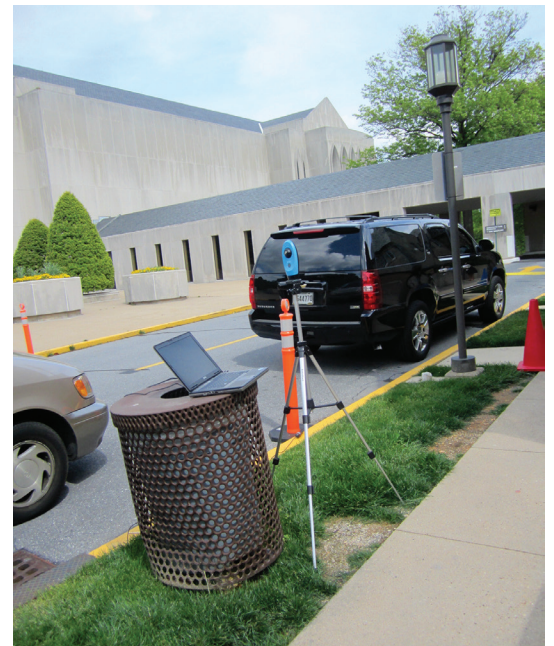
Figure 3. A laptop computer with two Vernier temperature probes and one CO 2 probe was set up in the carpool lane while a time-lapse camera recorded the arrival of cars.
